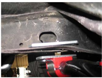
9. After drilling the holes, lubricate the swaybar bushing and reinstall onto swaybar. Using the hardware supplied install the bushing brackets and frame support plates (photo 6) one support plate between the bushing and the frame and the other inside and on top if the frame. Positioning the bolt with a washer on dropping down from inside the frame is easier. Attach bracket and then tighten all hardware.
