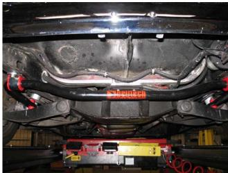
**10.** Check that all components and fasteners have been properly installed, tightened and torqued. Check brake hoses, and other components for any possible interference. Lift the vehicle and remove the support stands. Carefully lower the vehicle to ground.
