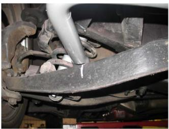
7. After drilling the holes, assemble the end links so the sway bar is in the correct position. (photo 4)
